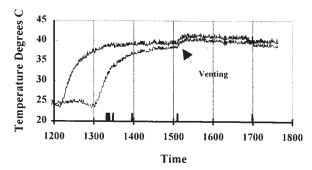
Figure 3. Temp. of side of roll during metallizing
