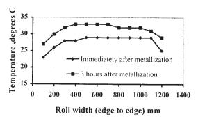
Figure 1. Temperature across width of metallized BOPP
