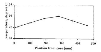
Figure 2. Temperature through depth of roll
